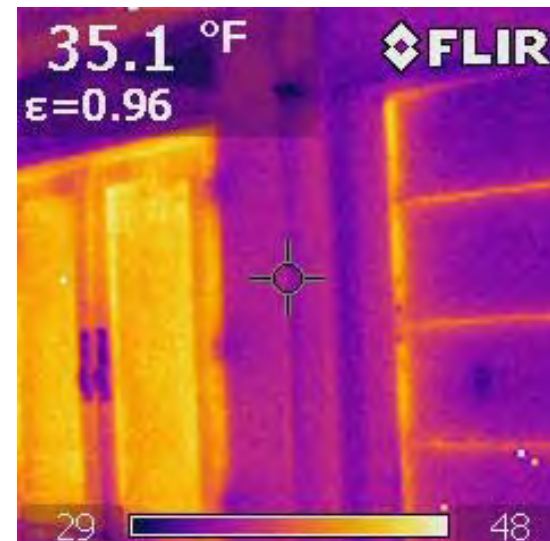
An infra-red image showing heat loss through a sliding glass door (left) and the garage door seams (right).
