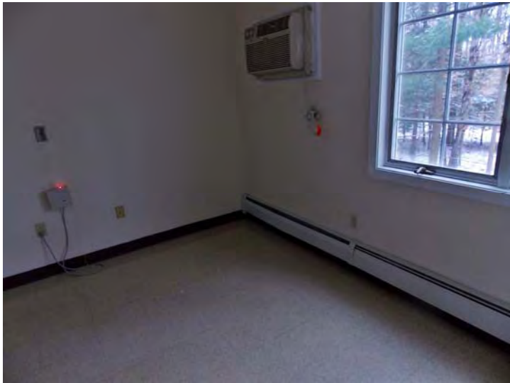
Each apartment has hydronic baseboard heat and a through-wall air conditioner sleeve. (Resident-owned air conditioner).
